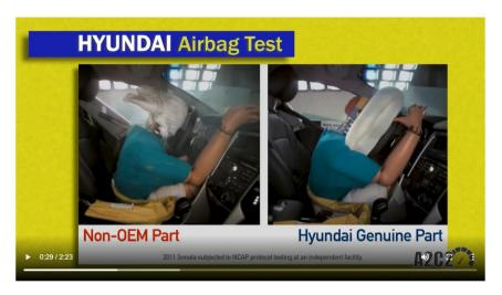
"In comparing genuine versus counterfeit airbags, all of the counterfeits failed to deploy in a proper manner. This shows how ineffective these potentially life-saving devices can be when counterfeited." Counterfeit Parts Testing | Automotive Anti-Counterfeiting Council (a2c2.com)
